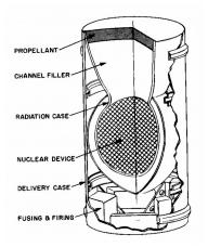
The configuration of the channel filler and propellant disc determines the angle of spread of the tungsten plasma. For propellant bombs, this should be wide enough that the entire pusher plate is in the cone, so that the energy density at each individual part of the plate is as low as possible. But it can be made much, much narrower, and pointed at something less resilient than hundreds of tons of steel pusher plate.
